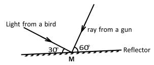
A ray from a bird makes an angle of  $30^{\circ}$  with a plane reflector and a ray from the barrel of a gun makes an angle of  $60^{\circ}$  to the same reflector at the same point, M as shown in figure **above**. Find the angle through which the reflector must be rotated about M such that the ray from the barrel of the gun falls on the bird.
