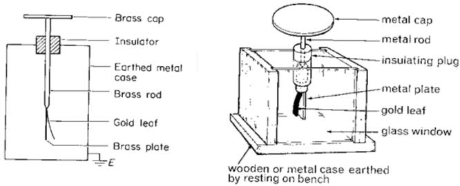
The gold-leaf electroscope consists of a brass cap and brass plate connected by a brass rod. A gold leaf is fixed together with a brass plate onto the brass rod.
