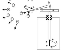
The pin placed on the cap of the positively charged GLE becomes positively charged as the GLE but with a high charge density at the sharp point.
