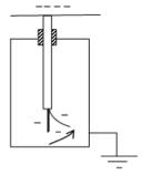
**NOTE:** In induction process, the electroscope acquires the opposite charge to that of the rod/body used to charge it.
