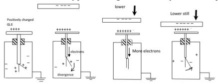
An electroscope is first charged positively.
