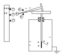
A needle is placed on the cap of an uncharged GLE to act as a sharp point. When a positively charged rod is brought near to the sharp end of the needle, the leaf rapidly diverges and stays diverged even when the rod is removed. On testing, the GLE is found to be positively charged.
