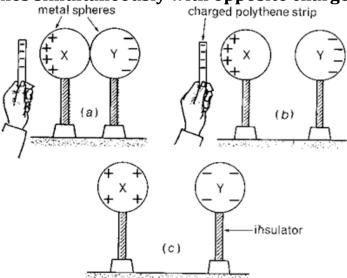
Two metal spheres X and Y that are mounted on insulated stands are placed in contact with each other as shown in (a)
