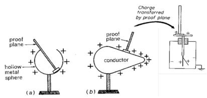
When the proof plane is placed on the outside surface of a charged hollow conductor mounted on an insulating stand, and then transferred to the cap of an uncharged G.L.E, the leaf diverges as shown in (a). This proves that charge was present on the outside of the surface.
