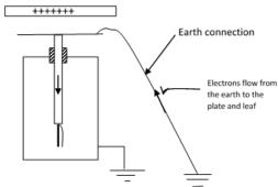
Electrons flow from the earth via the earth connection to the plate and leaf to neutralize the positive charge on them.
