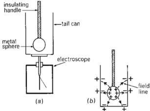
A metal pail is placed on the cap of an uncharged GLE.
