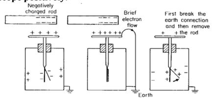
A negatively charged rod is brought near the cap of the gold leaf electroscope.
