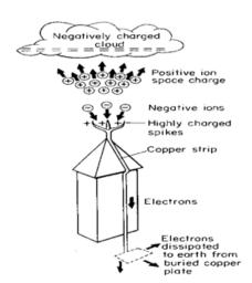
A lightening conductor is used to protect buildings from damage once struck by lightning by providing a path for electrons to flow easily through it.
