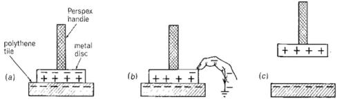
The slab of insulating material is charged negatively by friction.
