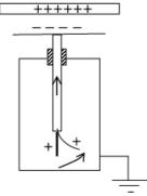
The gold leaf electroscope is then earthed momentarily in the presence of a positively charged rod by touching its cap.
