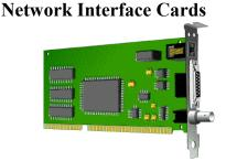
The network interface card (NIC) provides the physical connection between the network and the computer workstation. Most NICs are internal, with the card fitting into an expansion slot inside the computer.
