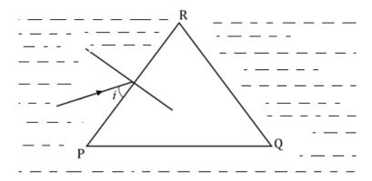
A ray of monochromatic light from a liquid of refractive index 1.3 strikes side PR of the glass prism of refractive index 1.6 at an angle  $i=70^{\circ}$ . Calculate the refracting angle of the prism for which the emergent ray from side RQ grazes the surface of the prism. (04 marks)
