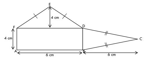
a) Determine the centre of gravity from AB and AF taken as the x and y axes respectively (state it as a coordinate).
