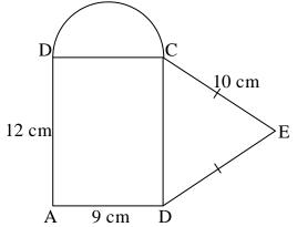
Find the position of the centre of gravity of the lamina from the sides AB and AD.
