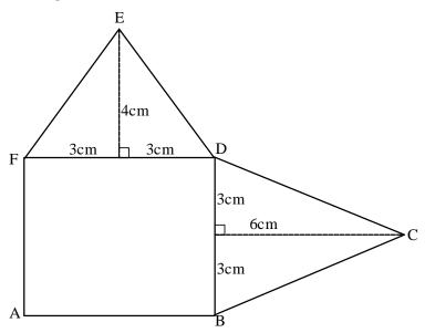
Determine the centre of gravity of the composite lamina ABCDEF from AF and AB taken as the y and x axes respectively. State it as a co-ordinate.
