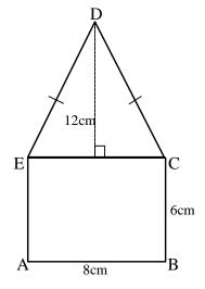
ABCE is a rectangle and DCE is an isosceles triangle with dimensions shown. Find the position of the centre of gravity of the complete lamina from AB.
