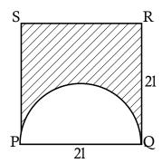
a) Show that the distance of the centre of gravity of the figure from PQ is  $\frac{201}{3(8-\pi)}$ .
