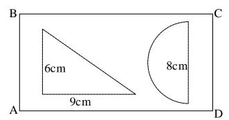
The straight side of the semicircular cut out is 1cm from the side CD and placed centrally between BC and AD. The perpendicular sides of the triangular cut-out are 2cm from the nearest sides of the lamina. Find the position of the centre of gravity of the remaining lamina.
