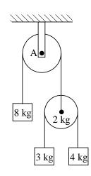
The system is released from rest. Determine the: Acceleration of the a) movable pulley, 3kg mass and 4kg mass. b) Tensions in the strings.
