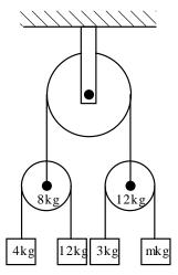
The acceleration of 4kg and 12kg masses are  $\frac{g}{2}$  upwards and  $\frac{g}{2}$  downwards respectively. The accelerations of the 3kg and mkg masses are  $\frac{g}{3}$  upwards and  $\frac{g}{3}$  downwards respectively. The hanging portions of the strings are vertical. Given that the string of the fixed pulley remains stationary, find the:
