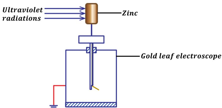
When Ultra violet light is incident on a clean zinc plate placed on the cap of a gold leaf electroscope:
