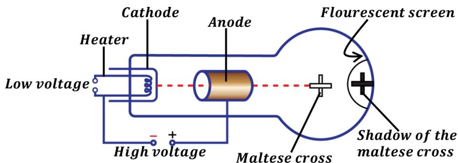
When cathode rays are directed towards the Maltese cross in a cathode ray tube. A shadow of the cross is formed on the fluorescent screen. The formation of the shadow verifies that cathode rays travel in a straight line.
