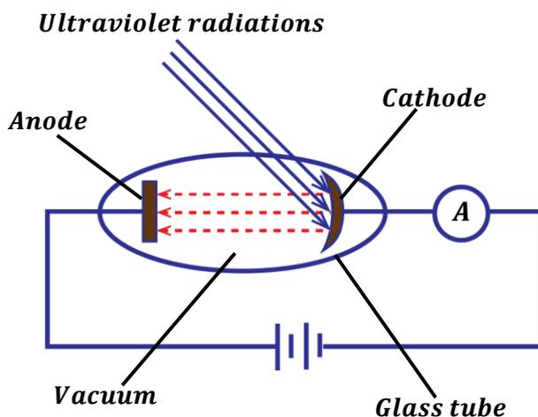
**Mechanism of a photoelectric cell:**
